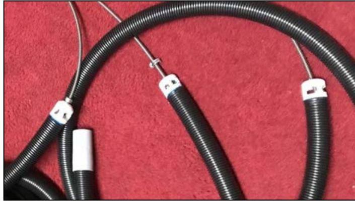
Figure 15—Final 1.25-in.-diameter hose configuration with plumber's snake.
