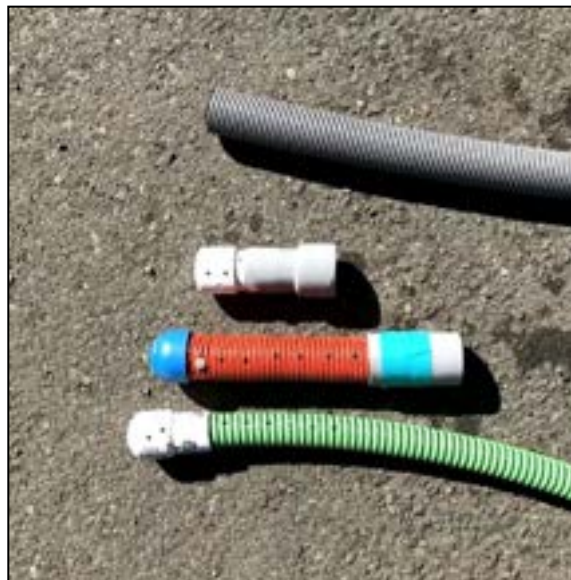
Figure 10—Hoses and tips used during initial testing. Perforations can be seen on the hoses.
