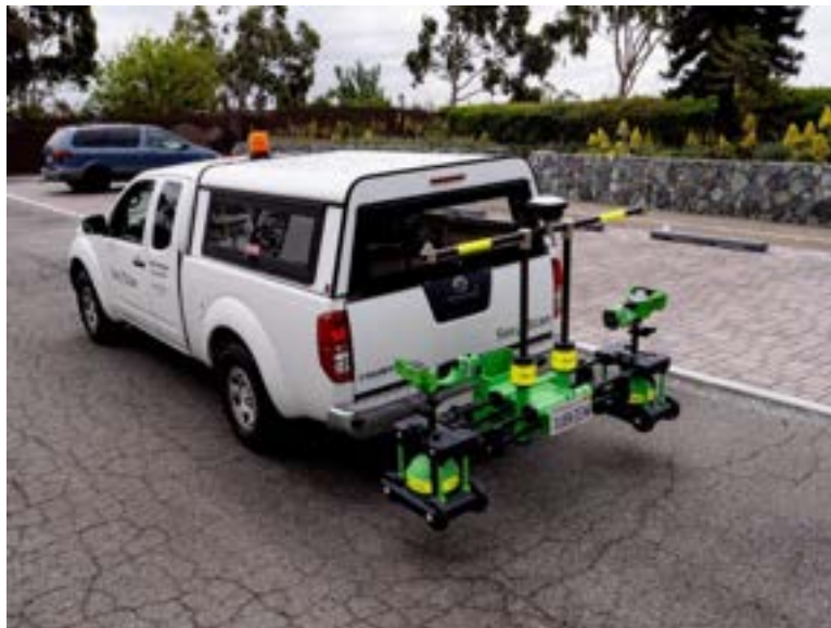
Figure 1—Geolocating receivers mounted to a custom vehicle hitch.
