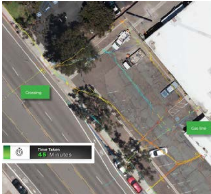
Figure 3—Zoomed in, the map data in SubView shows distinct utilities. Each line was energized with different groups of frequencies.
