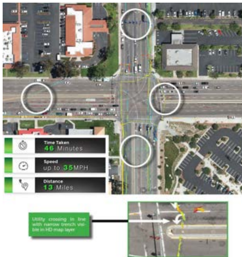
Figure 2—The intersection shows the density of signals detected at various depths, revealing the presence of multiple utilities that cross the intersection.
