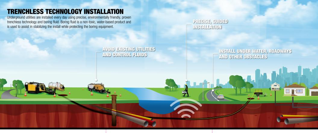
**Trenchless installation equipment** is used to tunnel underground and install utilities with minimal ground disturbance. Trenchless installation is a proven method that has existed for over half a century. It is environmentally friendly and offers a lower carbon footprint than other installation methods. It also produces less noise pollution.
