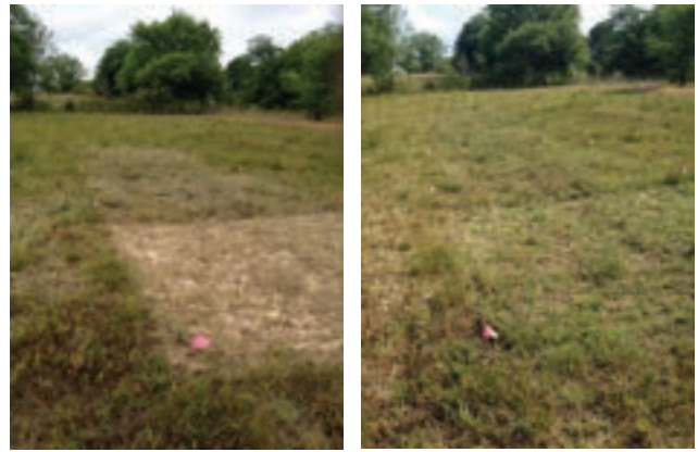
Figure 3. Picture of several established Bermudagrass plots immediately after application of HDD mud (left) and seven days after application and nearly three inches of rainfall (right).
